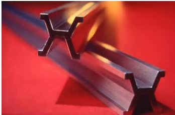
Figure 9: Platinum-Iridium meter bar [9]
